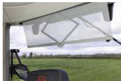
SUN SHADE - Up to four sun blinds, along with the tilted front windscreen and the large roof, provide shade for total protection.
