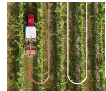
▲ SPEEDSTEER reduces operator effort for faster operation on the headland and it enables the operator to adjust the steering ratio.
