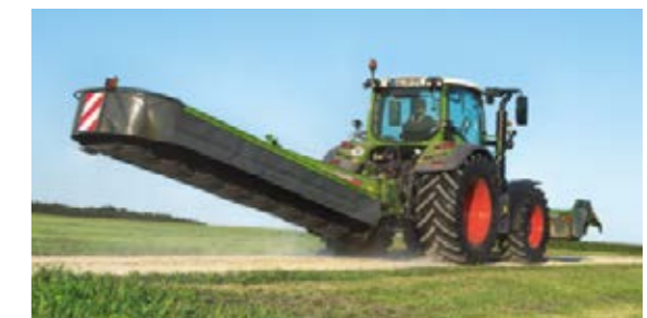
The mower swings through 90° to the rear from the cab in the transport position.
