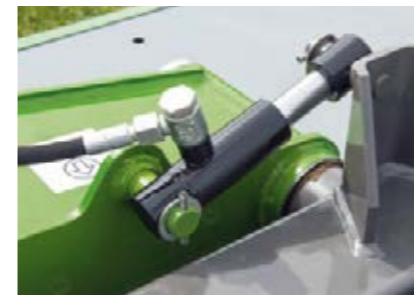
The compensation cylinder stabilises the mower unit on headlands and on the roads.
