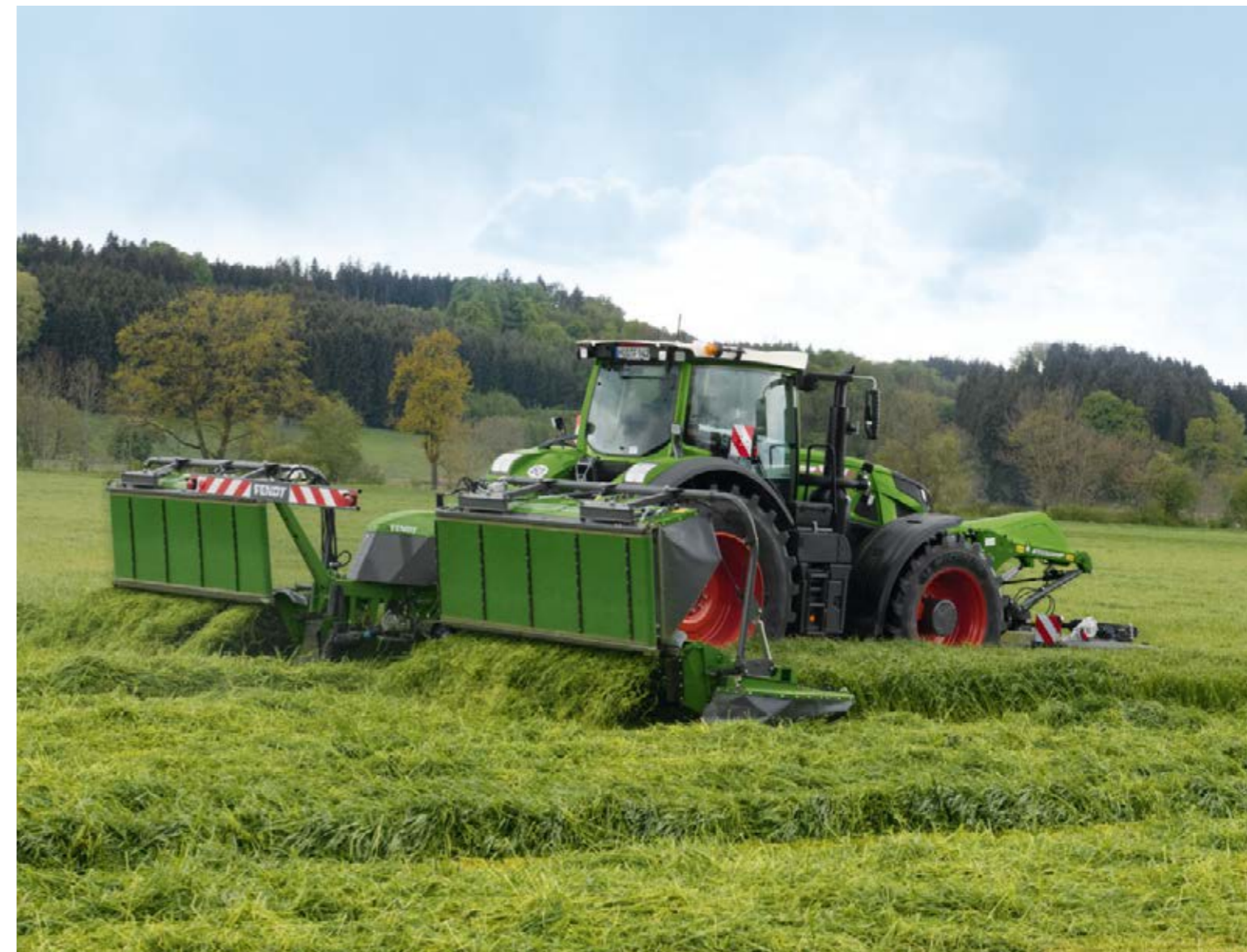
The belts can be folded up and the crop discharged across the full width at the touch of a button.
