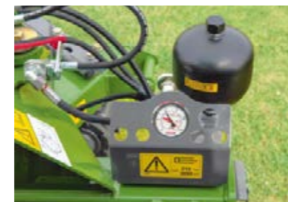
The hydropneumatic TurboLift cutterbed relief enables a single, floating cut.
