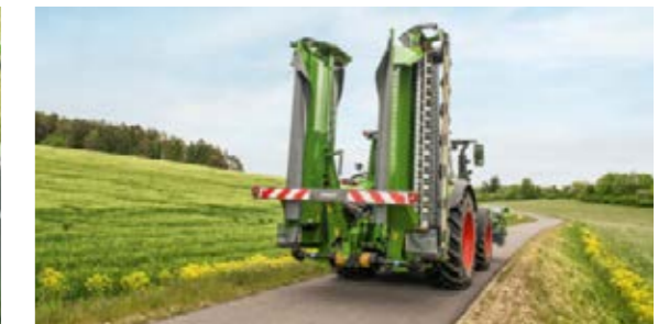
When folded, the mower combination remains below 4 m in height, and can be easily driven thanks to the low centre of gravity.
